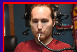
- Head Array Drive System (primary method) - Sip-n-Puff Drive System (secondary method for bumpy and un-even terrain)
