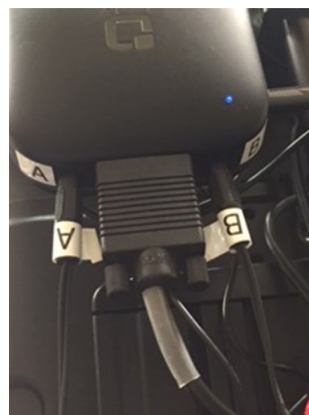
Figure 6. 1/8" (3.5mm) Mono Male-to-Male 6 ft. cables were connected to Tecla-E Ports 'A' & 'B' for accessing iOS devices from bed using custom-designed sip-n-puff switch. Mono cables are long enough that Tecla-E can remain mounted to chair.
