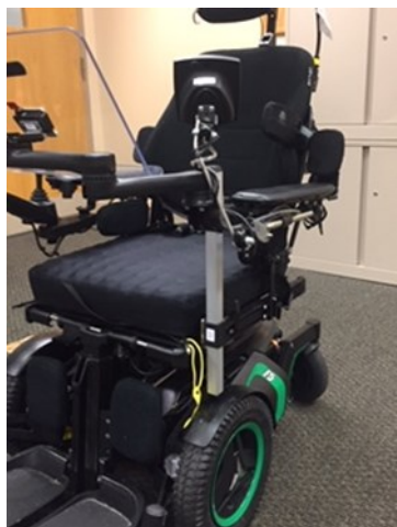
Figure 1. Permobil F5 Corpus VS standing power wheelchair with Moun't'n Mover Easy Mover Dual Arm with Quick Connect plate, low-resistance hinge, and clear tray with lip by BlueSky Designs. iOS devices secured to tray with Velcro
