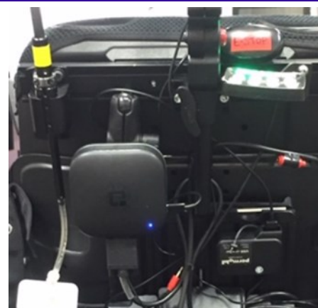
Figure 5. Permobil USB Charger powering Tecla-E via USB C cable. Tecla-E is accessed via profile/Mode 5 (programmed as an output module).
