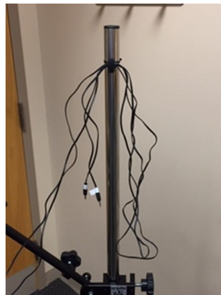
Figure 10. Mono cables are removed from inputs 'A' and 'B' of Tecla-E (when Mike is not using his devices in bed) and are secured to CJT floor mount pole. Additionally, Enabling Devices switch is removed from Mount'n Mover tray and clamped to adjustable arm of ET Roller.
