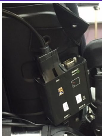
Figure 3. R-Net Input/Output Module (IOM) connected to power source and attached to Tecla-E via 9-Pin (DB9) Male-to-Female Serial Port Cable.
