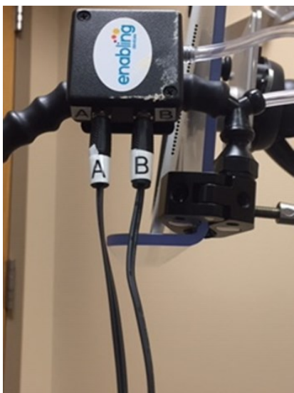
Figure 8. Enabling Devices Easy Flex Sip-n-Puff Switch clamped to Mount'n Mover tray with switch inputs 'A' and 'B'.
